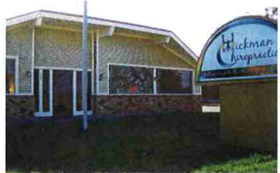
Dr. Hickman's office utilizes awnings to help control the amount of heat from sun light to manage AC costs.
